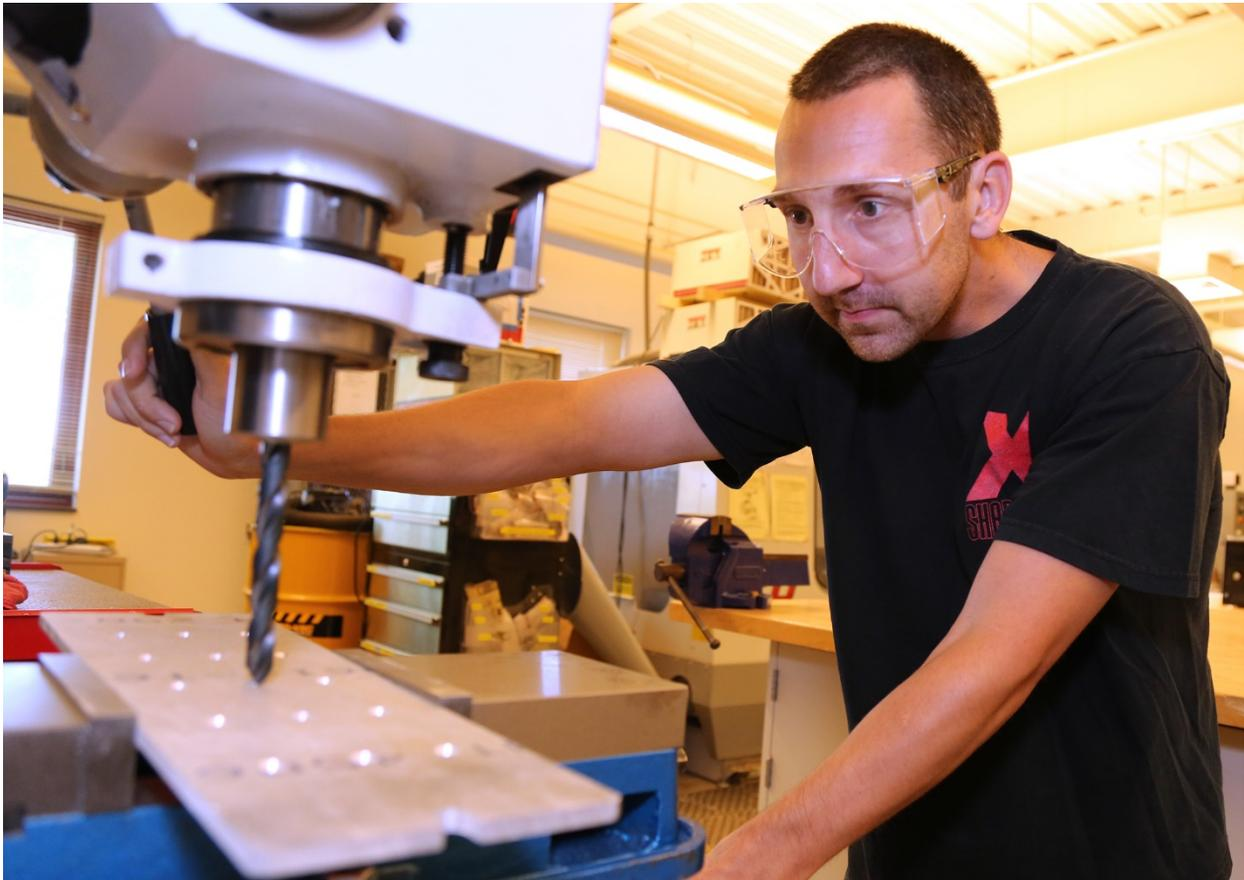
Jason Boyer, 39, of West Mifflin, Allegheny County, a student in Butler County Community College's manufacturing pre-apprenticeship certificate program held on BC3's main campus in Butler Township, locates a drill to a piece of metal using a digital readout on a geared milling and drilling machine in BC3's manufacturing lab on Monday, July 15, 2019.
